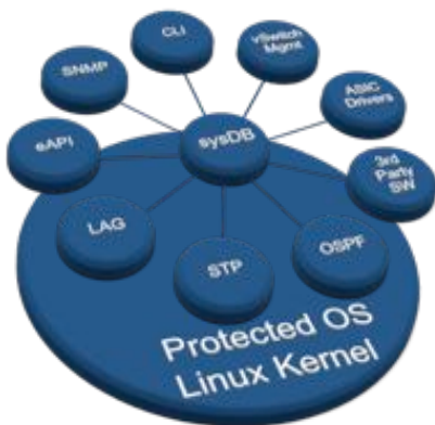
Figure 20: Arista EOS Software Architecture showing some of the Agents
